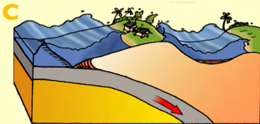
When the islands suddenly rise, water flows away from the land, but it comes back as a series of ocean waves, called tsunamis.
