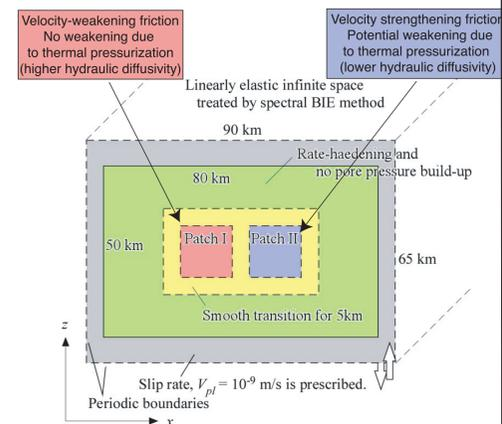
Fig.10: Model Set-up (Noda and Lapusta, JGR 2010, in prep.)
