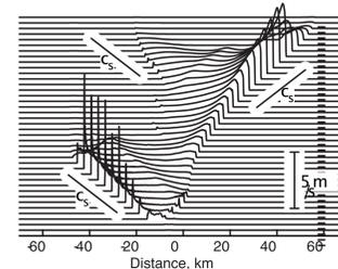
Fig.14: Snapshots of slip rate of the 26th event (Noda and Lapusta, in prep.)
