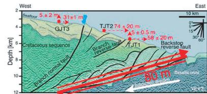
Fig.2: Pre-existing seismic structure and observed deformation of the frontal wedge (Tsuji et al., EPS, 2011). Red arrows indicated the observed displacements from Ito et al., GRL 2011.
