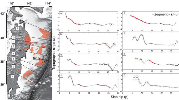
Fig.7: left: Critical mechanical areas where internal and basal friction and fluid pore pressure can be inferred. right: Mean +/- sigma of the taper for each segment, critical accretionary prism in red.
