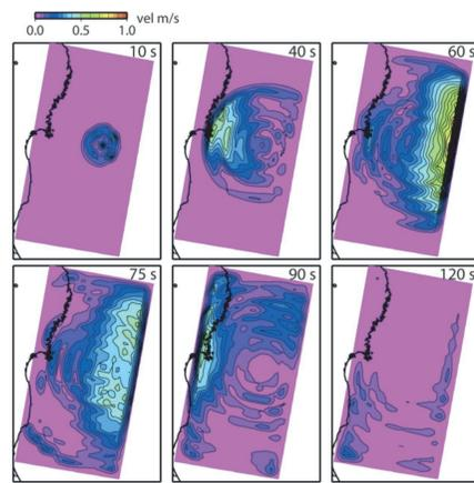
Fig.4: Snapshots of the slip-rate distribution at 6 times from Ide et al., Science 2011.
