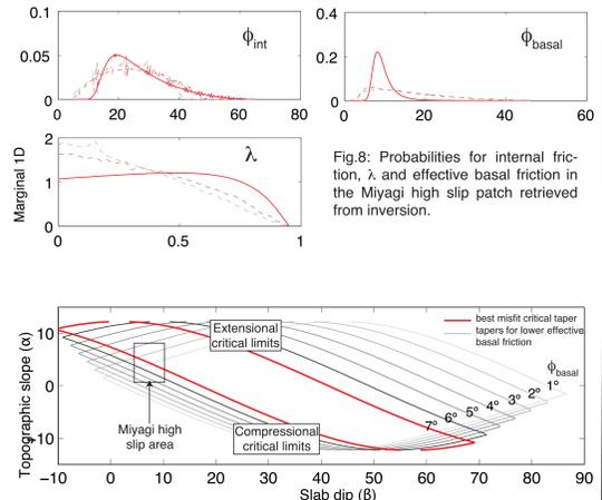
Fig.8: Probabilities for internal friction, lambda and effective basal friction in the Miyagi high slip patch retrieved from inversion. Fig.9: Critical envelopes for basal friction (phi\_basal) ranging from 1 to 7 degrees, with lambda=0.8. In red: critical envelope for values of the best misfit. A decrease of 5 degrees could lead to normal faults activation.
