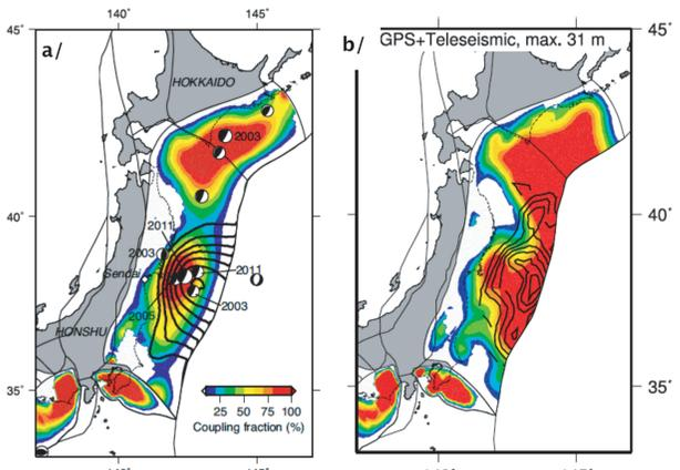
Fig.3: a/ Pre-Tohoku-Oki earthquake coupling model with no interseismic strain accumulation on the up-dip and down-dip edges, b/ Relaxing the assumption of zero interseismic coupling along the Japan trench from Loveless and Meade, GRL 2011.
