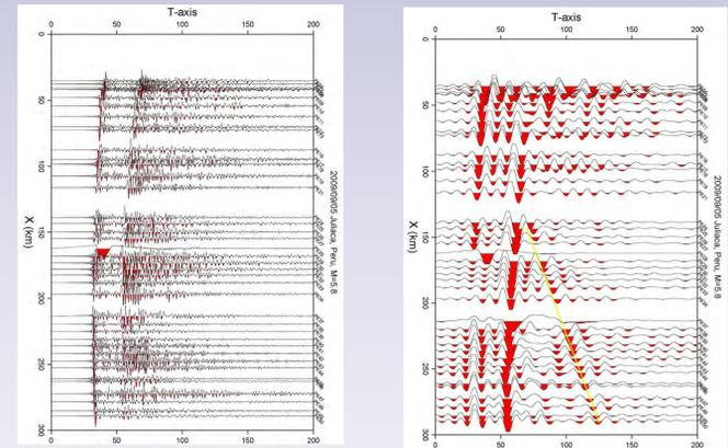
Juliaca earthquake, M 5.8 on Sept 5, 2009. Left is data banded to 1s, right at 10s. Signal observable in 10s data which may be a surface wave reflection (yellow line) off of corner where slab meets the Moho or topography
