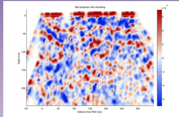
Backprojection image of teleseismic receiver function data
