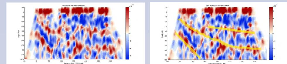
Above: Receiver function image of the lithosphere in Southern Peru. On the right is a possible interpretation of the results in which the middle line (thickening to about 70 km beneath the Altiplano) is the current Moho depth, the line at about 40 km is a mid-crustal structure, and the third line is the subducting slab
