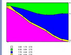
Above: P-wave speed model used in Finite Difference code. Crustal thickness based on receiver function results, slab dip of about 30 degrees based on teleseismic and PKP
