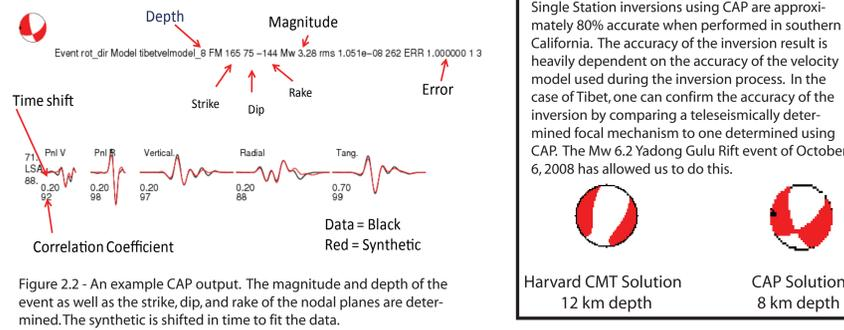
Figure 2.2 - An example CAP output. The magnitude and depth of the event as well as the strike, dip, and rake of the nodal planes are determined. The synthetic is shifted in time to fit the data.
