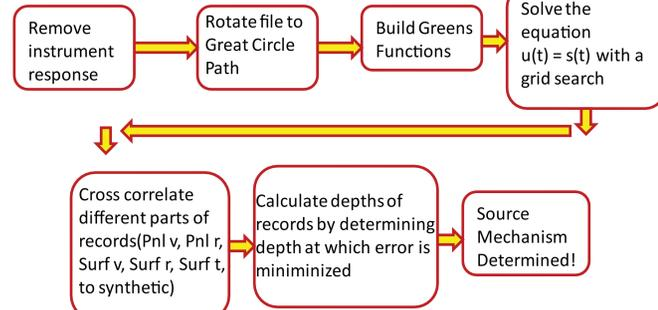
Figure 2.1 - Flow chart illustrating the steps in the CAP method.
