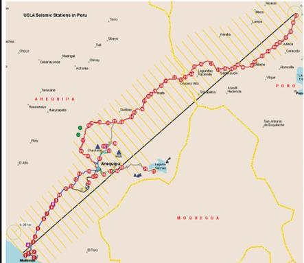
Above: Seismic array of 50 broadband seismic stations installed with 6 km spacing.
